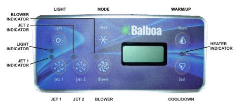
**Default System Operation:** When power is applied, or there is a loss of power the system will initiate its default programming. The filter cycle will start 6 minutes after power has been applied and repeat 12 hours later if programmed to do so.
