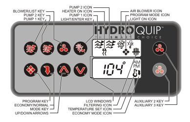
**Default System Operation:** When power is applied, or there is a temporary loss of power, the system will initiate its default programming. The filter cycle will begin 24-hours after the system has been powered up. The filtration cycle will be active for 1-hour and will repeat every 24-hours. The temperature will be maintained at 95°F.
