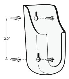
Note: If the cradle is mounted onto a wood surface, inserts and a pilot hole may not be necessary.
