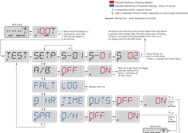
\*If the Control Panel does not have a Warm (Up) button, but rather a single Temp button, use the Temp button in place of the Warm button in the instruction above. (The flow chart assumes a single Temperature Button.)
