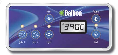
VL701S (Serial Standard) PN 51247-01 with Overlay PN 10402 • Connects to Main Board terminal J1 only\*
