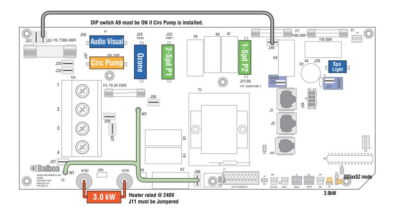
WARNING: Main Power to system should be turned OFF BEFORE adjusting DIP switches. WARNING: Persistent Memory (J43) must be RESET to allow new DIP switch settings to take effect. (See Persistent Memory page)
