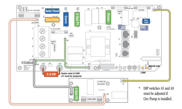
**WARNING:** Main Power to system should be turned OFF BEFORE adjusting DIP switches. **WARNING:** Persistent Memory (J43) must be RESET to allow new DIP switch settings to take effect. (See Persistent Memory page)
