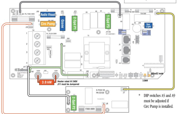
**WARNING:** Main Power to system should be turned OFF BEFORE adjusting DIP switches. **WARNING:** Persistent Memory (J43) must be RESET to allow new DIP switch settings to take effect. (See Persistent Memory page)
