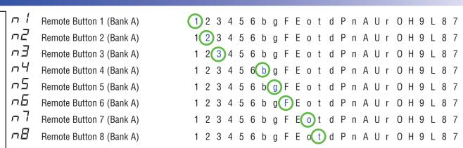
1-6 = Assigns Pump Number (Pump 1, Pump 2, etc); b = Blower; g = Spa Light; F = Fiber-Optic wheel/light; E = EitherLight;
