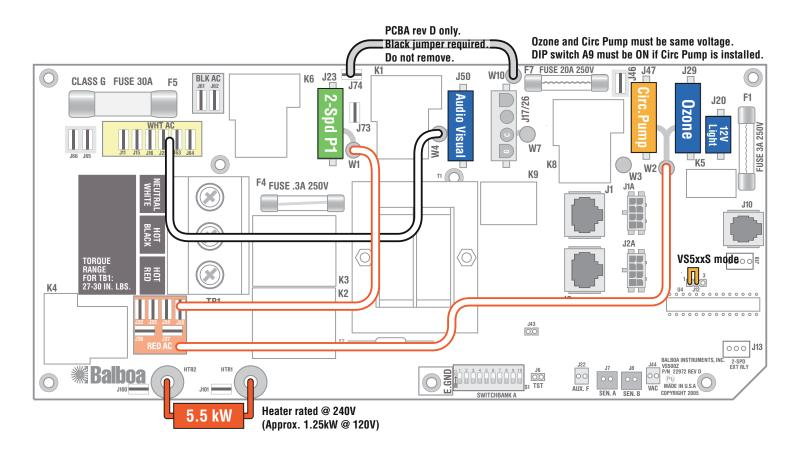
WARNING: Main Power to system should be turned OFF BEFORE adjusting DIP switches. WARNING: Persistent Memory (J43) must be RESET to allow new DIP switch settings to take effect. (See Persistent Memory page)
