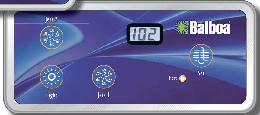
VL402 (LCD Duplex Digital) PN 54107 with Overlay PN 10764 • Connects to Main Board terminal J1 or J2 • Not compatible with some configurations; not recommended for new designs
