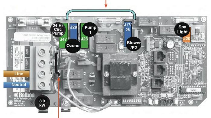
Single Service Connection Shown Above - One 16 Amp or One 32 Amp Service. For 32 Amp service, DIP Switch A10 may be changed to the "High Amp" setting.
