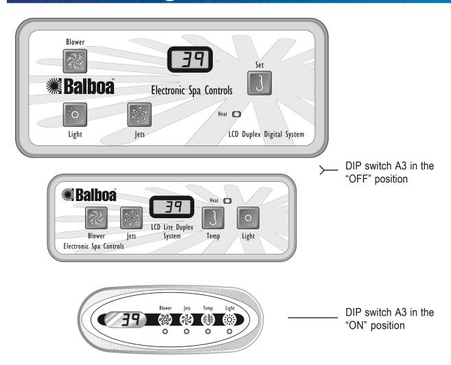
Several configurations of the panels above can be created as custom parts. Separate Temperature Up and Down buttons can be done if no Blower is present. Jets 2 button available if no Blower is present.
