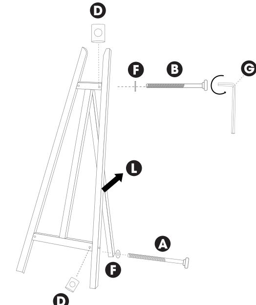
**ENG** Fit part L into assembled unit as shown. Secure using bolts A, washers and cams. Now tighten all bolts using allen key.
