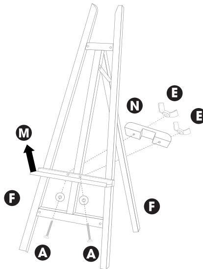
**ENG** Attach the canvas support M and N to the assembled unit as shown. Secure using bolts A, washers and wing nuts, but do not over tighten the bolts.
