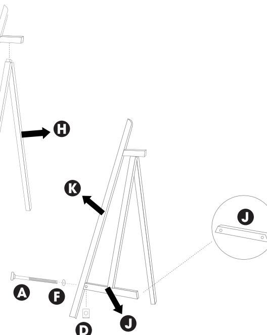
**ENG** Fit part H into assembled unit as shown. Fit part J into assembled unit as shown. Secure part K and J, using bolt A, washer and cam. Do not tighten bolt at this moment.
