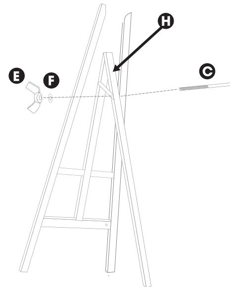
**ENG** Secure Support H, Using Bolt C, Washer and wing nut, but do not over tighten the bolt. Assembly is now complete.
