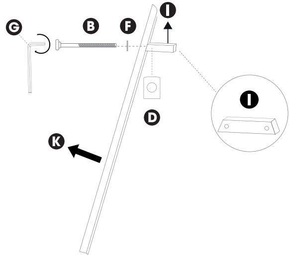
**ENG** Assemble part K and I, using bolt B, washer and cam. Do not tighten the bolt at this moment.
