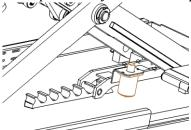
b. Use a wrench to loose the core of the electro-magnetic valve to lower the platforms.
