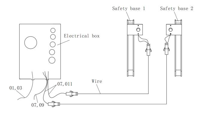
01,03——the limit switch wiring; 07,11——the electromagnet wiring; 07,09——the electric release valve
