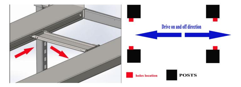
Recommendation:Our lifts are designed and manufactured in perfect performance,but wax the outside of the posts with paste wax or spray wax can reduce friction and keep smooth operation. Do not recommend to use grease,which will make it dirty.
