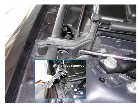
5. Align the harness into the wire bridge and attach the black ground wire. You will need a 5/32 allen wrench for the screw provided.
