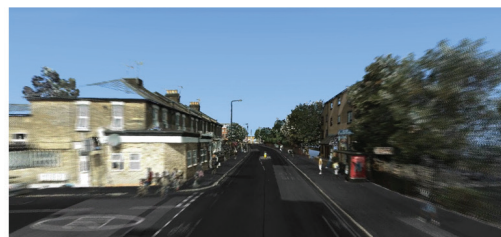
Ladybug imaging mapped to LIDAR point cloud
