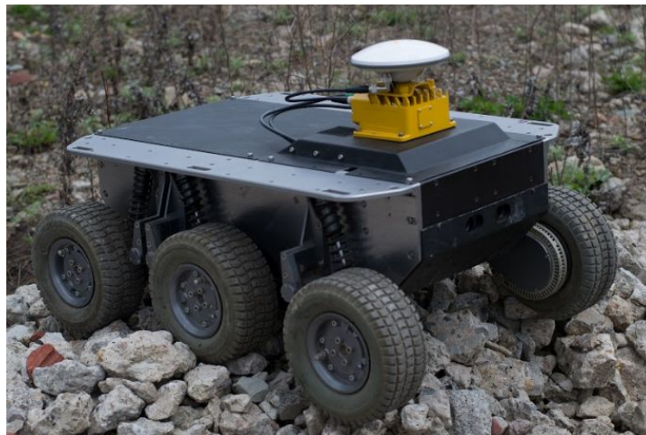
Figure 1: Duro Inertial sample mounting
