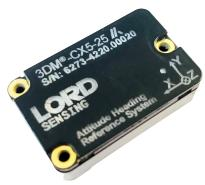
3DM-CX5-25-high-performance, industrial-grade attitude and heading reference system (AHRS) with integrated magnetometers, high noise immunity, and exceptional performance
