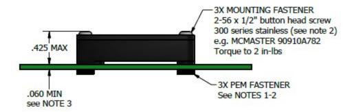
NOTE 1: For solderable fastener: PEM p/n SMTSOB-256-2ET see product datasheet for details. Alternate: 0.067 thru (with or without copper pad) for conventional nut mounting (see note 2).
