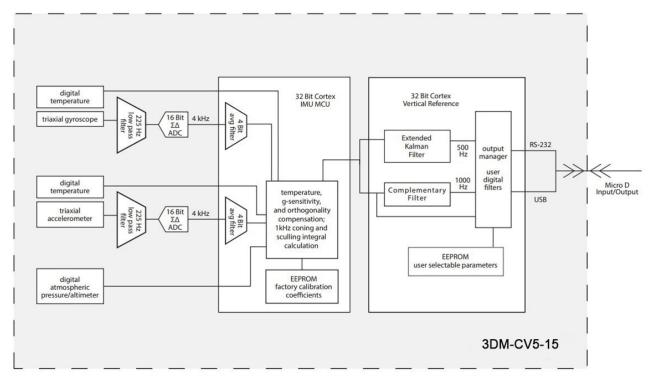
Figure 14 -3DM-CV5-15 Block Diagram
