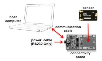
Figure 5 -System Connections
