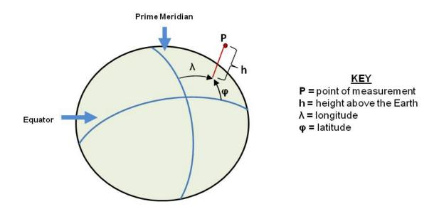
Figure 17 - World Geodetic System (WGS84) Reference Ellipsoid
