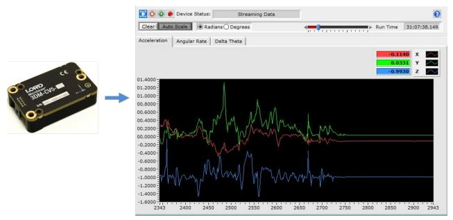
Figure 3 -Viewing Sensor Data with MIP Monitor
