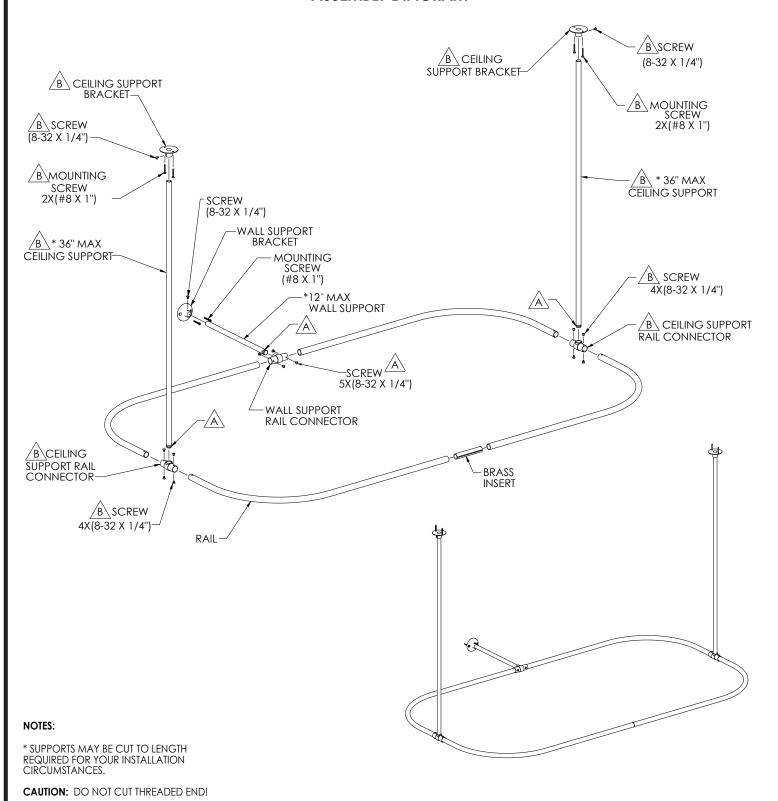
THREADS ON PIPES ARE SHALLOW THREADS. DO NOT OVERTIGHTEN
