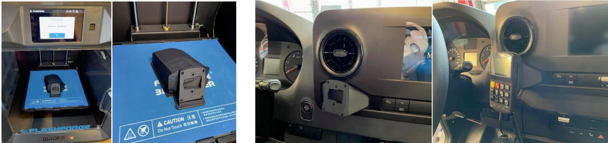
Display of the printed placing bracket of the radio equipment controller and its practical application
