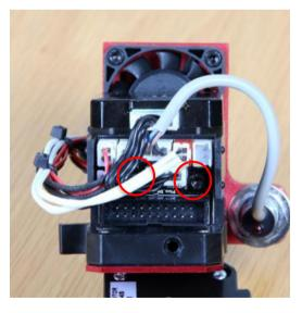
• Locate the two M3 screws that holds the board to the carrier.
