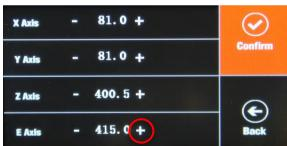
Press the + sign for E Axis until the value is changed to 415
