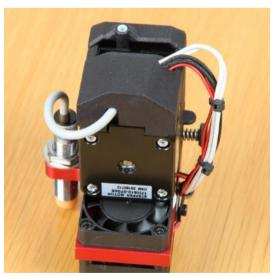
• And the cut-out for the inductive sensor on the rear side.
