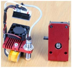
• Slide the extruder off the bottom plate and put it aside.
