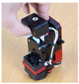
Place the extruder assembly on a flat surface and remove the cover over the breakout board.
