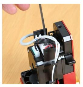
And remove the 2 screws using a 2,5mm hex wrench.
