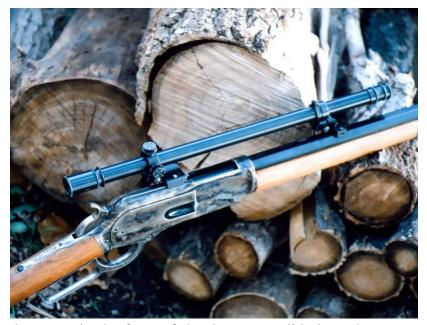
The base set consists of a front and a rear base. The front base replaces the rear sight and all that is required is to remove the rear sight and then install the dovetail block of the front base. Once the block is centered in the dovetail slot, the base screws are installed and tightened.
