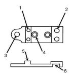
block and tighten the two screws from the base into the block. Use the existing hole (3) and drill and tap two 8-40 holes as (4) indicates. Screw the base on the base and lock-tite the screws on the base. After you secure the heavy-duty base, then mount the rear scope mount on top (5). See the mounting details in the scope instruction manual. If you have any questions about this product, please feel free to contact us at the toll free no. 1-888-HI-LUX-12 (445-
