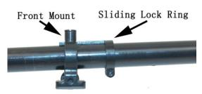
Insert the spring and tighten the cap screw slowly. Meanwhile, you need to check and see the front mount can be moved back and forth smoothly. Make sure the reticle is straight and tighten the sliding lock ring screw to prevent the front mount moving.
