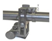
Install the TLC to fit against the back of the rear elevation block as the photo shows. You can remove the E.P. from the back quickly and slide the TLC on the tube and put the E.P. back on as soon as you can. You should tighten the two screws on the TLC tightly. Now the scope should not move forward during shooting. (If the TLC is already on the tube, you just need to tighten the two screws).
