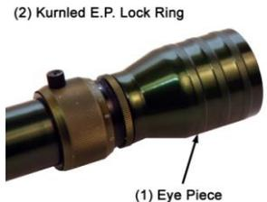
focus. After you get a sharp reticle image, you can tighten the knurled E.P. Lock Ring by turning the knurled E.P. lock ring (2) counterclockwise to lock up the E.P. If you want to loosen E.P., you can either turn the E.P. (1) counterclockwise or turn the the E.P. knurled lock ring (2) clockwise.
