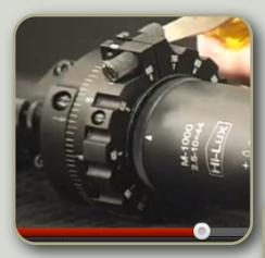
Once the CAM Ring is loosened, you can turn the CAM setting to match the correct setting for you round. In this picture, you will see the setting is 460.
