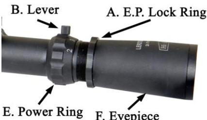
If the reticle is not sharply defined instantly, you need to change the scope's focus to suite your individual eyesight. Loosen the E.P.Lock Ring (A) (turn clockwise), and turn the Eyepiece (F) counter-clockwise or clockwise until you are comfortable with the focus. Then tighten (turn 4
