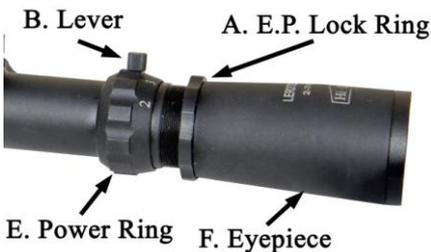
If the reticle is not sharply defined instantly, you need to change the scope's focus to suite your individual eyesight. Loosen the E.P.Lock Ring (A) (turn clockwise), and turn the Eyepiece (F) counter-clockwise or clockwise until you are comfortable with the focus. Then tighten (turn
