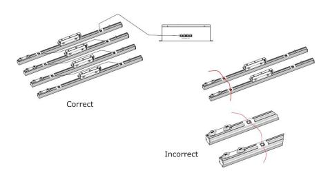
NOTE - When hanging multiple end-to-end connected fixtures vertically, be sure to secure each fixture together with safety cables. First, attach a safety cable from one fixture's hanging bracket to a secure rigging point. Then, secure each fixture together by attaching a safety cable from each fixture's mounting bracket to its neighboring fixture's safety cable loop.
