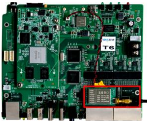
Figure 3-4 Install the Lora Device on Taurus of T6 Model
