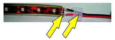
Insert the connector wires through the end cap, and solder the wires to the pads.
