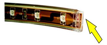
After the strip is cut, carefully cut and clear here to assure that there is enough space for soldering ribbon connector wires.
