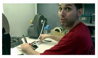
Marcus cutting a Super 8 film with the German made Würker tape splicer.
