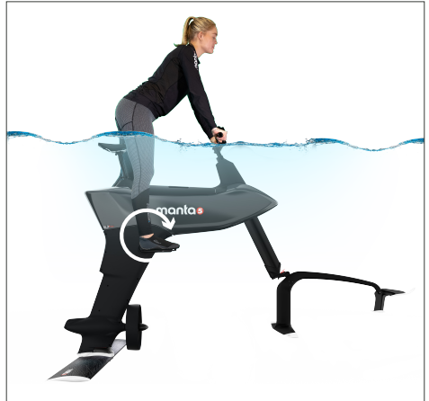
7.2 Stand on the pedals whilst staying in an upright position and rotate the pedals one full rotation (or press the activate motor button) to activate the motor, allowing the throttle to become active.
