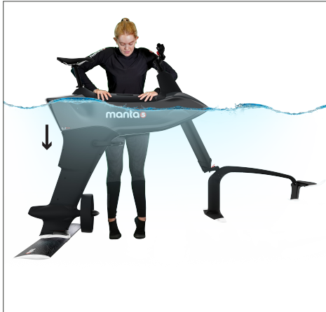
7.1 At a minimum depth of 2 meters, place your hands on the chassis and push the bike down under the water keeping it upright. Push the handlebars and seat down to sink it further while you climb on top of the bike.
