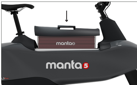
5.3 Insert the battery into the tub with the handle arrows pointing towards the front of the bike.
