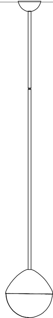
1. Place bracket on ceiling. Mark holes with a pencil. (lamp orientation can be adjusted later)
