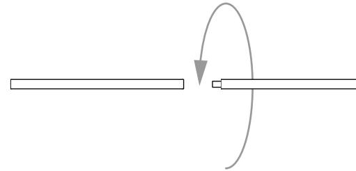
4. Thread wiring through the assembled rods and ceiling rose. Screw to the rod into the pendant and ceiling rose. (keep wire from twisting)
