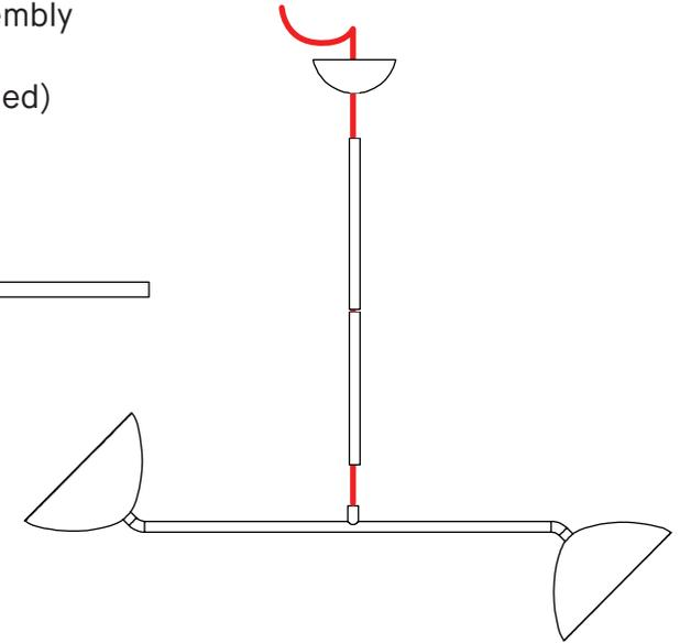
5. Once the lamp parts are all screwed together, the ceiling rose can be rotated so that you can choose the direction the pendant points in relation to the fixed ceiling bracket. (do not try to rotate lamp once it has been fixed to ceiling)
