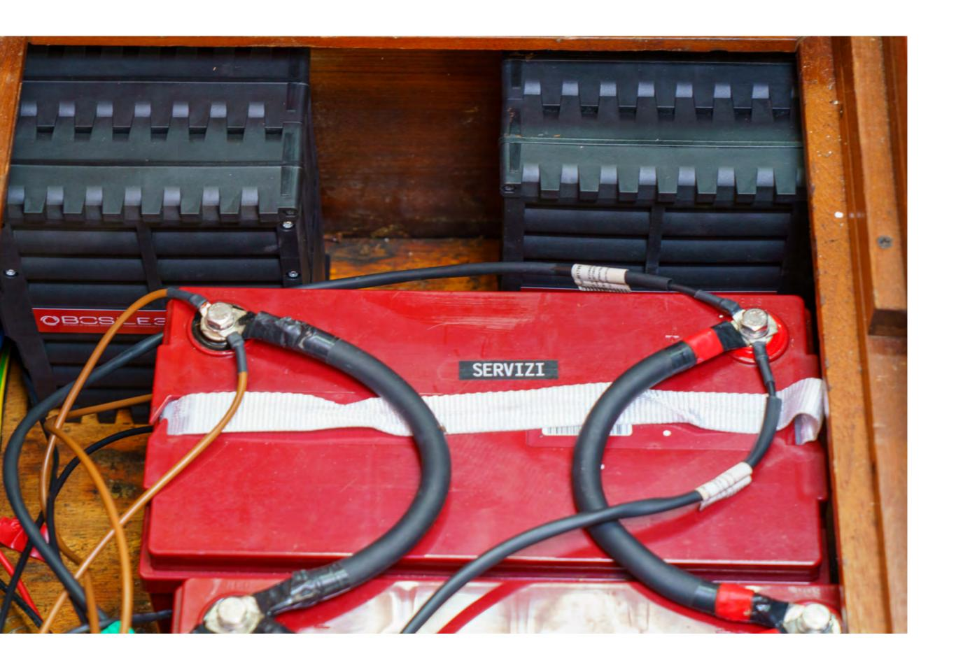
In place of the fifth battery, we will instead install 4 BOS LE300 modules which, as well as optimizing the operation of our energy reserve, will provide us with a total of 102.4 Ah and will be able to deliver 50 A of current, the AGMs will therefore only be "stressed" once this reserve has been used up.
