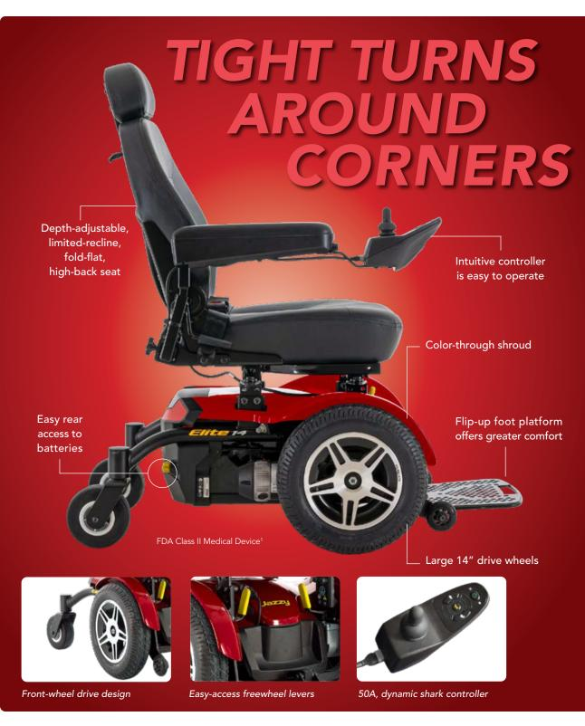
The Jazzy<sup>®</sup> Elite 14<sup>1</sup> is designed for excellent indoor maneuverability and outstanding outdoor capability. Featuring 14" drive wheels for enhanced outdoor performance combined with a front-wheel drive design to provide tight turns around corners. Large front wheels offer extra absorption over obstacles for superb climbing capabilities along with front anti-tip wheels for transitioning over grade changes and handling various terrains with ease.
