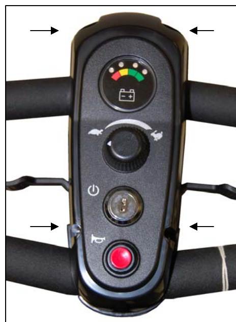
Figure 37. Control Panel Removal
