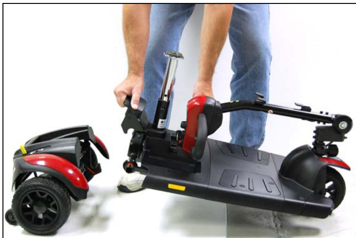
Figure 17. Separating the Drivetrain and Frame
