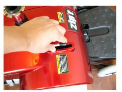
Step 2 Twist the two chrome release levers so that they are pointing forward.
