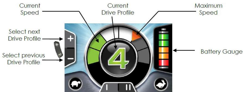
The operation of the function keys is dependent on the value of the [I II] Function Button
