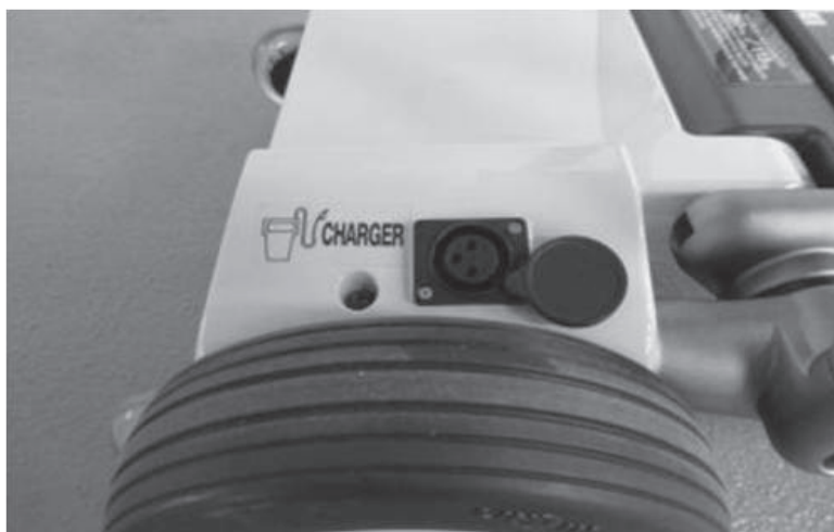
battery charging Port
