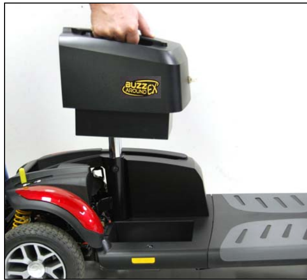
Figure 21. Battery Pack Installation
