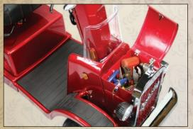
Front "under the hood" storage compartment with lock and key (tools not included).
