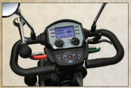
Intuitive digital display with dial-a-speed control, odometer, high/low gear differential, and dual option thumb/finger throttles.
