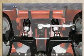
All wheel coil spring suspension system for a smooth ride at any speed.
