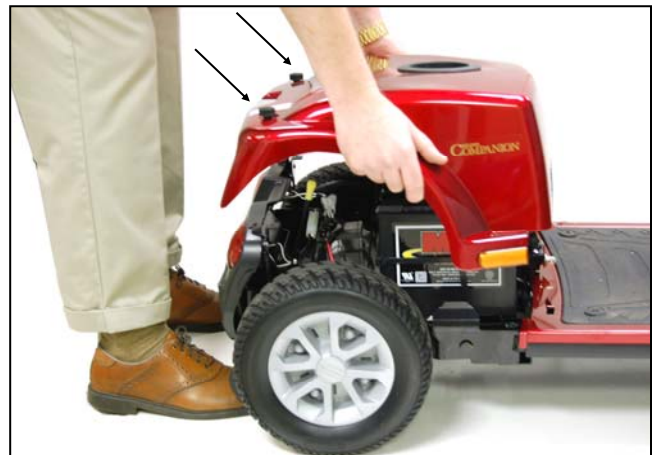
FIGURE 16. REMOVING THE REAR SHROUD
