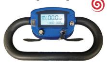
The informative LCD Display shows the battery level, battery voltage, speed you are traveling at and distance.
