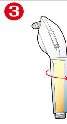
**Attention: Check the right direction to insert before loading the filter.**
