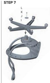
Insert the stand into connector, press hard (or press with a hammer), then add the cover plate onto it and use the screw sets to affix it.
