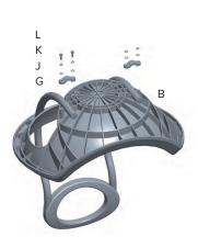
Use tube fixers and screw sets to fix bars on the chair base bottom. Fasten screw sets.
