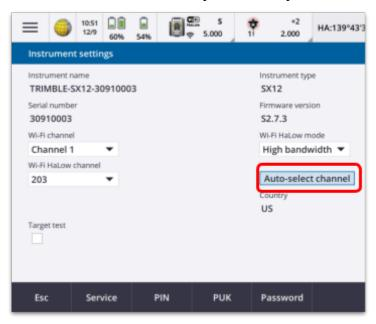
Since the Wi-Fi HaLow radio operates in license-free ISM band, it is possible that other radio devices that use the ISM band cause interference issues which could be perceived by laggy video when the signal bar in the application indicates a strong signal.
