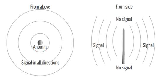
To get good radio range it is therefore important that both the Trimble EM130 and SX12 antennas are oriented in the same direction. As the Trimble SX12 antenna is fixed in a vertical position, make sure to position the tiltable antenna on the EM130 in the same vertical position to help achieve maximum range.
