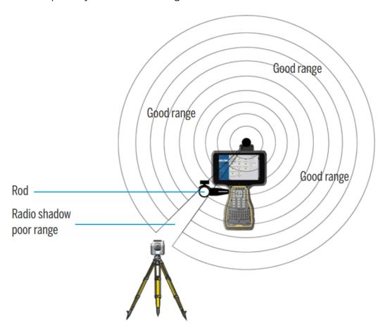
If the data collector has more than one Empower module bay, Trimble recommends mounting the EM130 module on the bay *farthest* from the rod to help mitigate this effect. Moreover, if you experience radio issues, try rotating the rod to allow for a clear line of sight.
